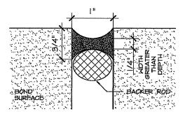
3 Detail 1; Clarification, Mortar Joint replacement is included in addition to unit quantities noted above.
